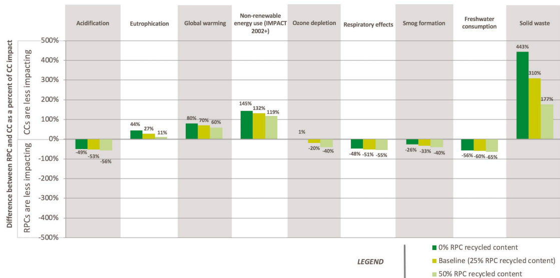
Figure 5-8. Sensitivity of RPC results to recycled content for RPCs containing apples. A positive value indicates CCs are preferable, while a negative value indicates RPCs are preferable.
